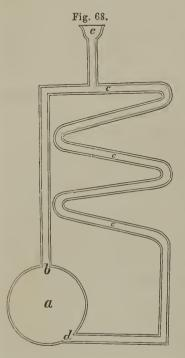
the mouth of the tube through which the hot water is distributed, c c the tube as it ramifies through the building, inclining, after it has passed a certain point, toward the boiler, and emptying into it at d; at e a tube is shown by which the air is allowed to escape from the water.
